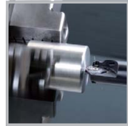
• Application on turning machine. Insert type no need to reset the tool length when changing.
