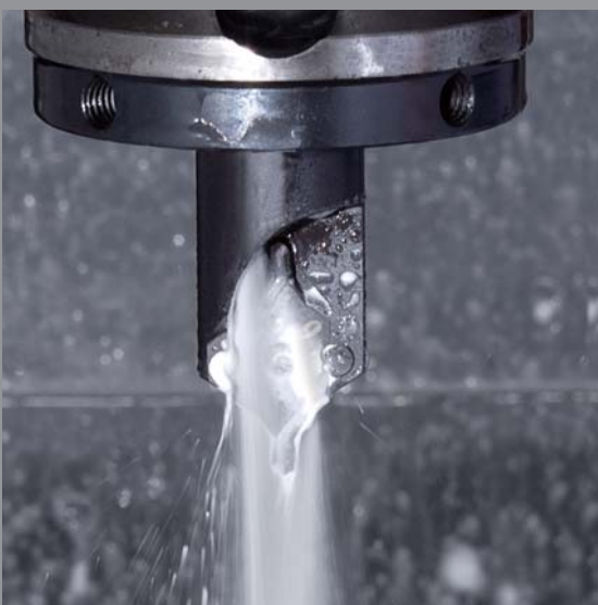
• Coolant supply from center
